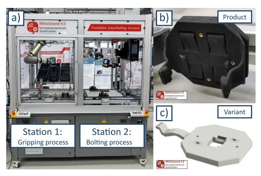
Figure 2: Picture of the assembly line with its two stations (a), the produced device holder (b) and a variant of the device holder (c).
