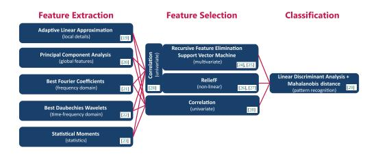
**Figure 4:** Algorithms of the automated ML Toolbox for classification with their corresponding literature (adapted from [6]).
