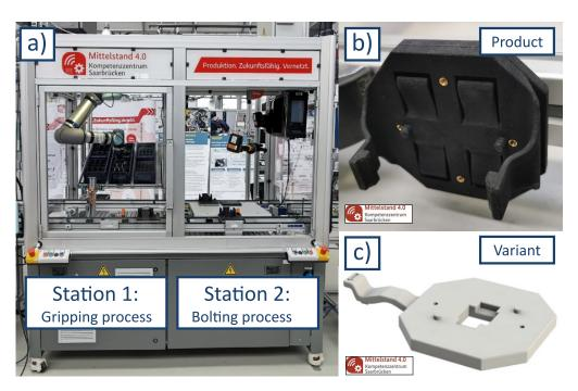
**Figure 4:** Picture of the assembly line with its two stations (**a**), the produced device holder (**b**) and a variant of the device holder (**c**).
