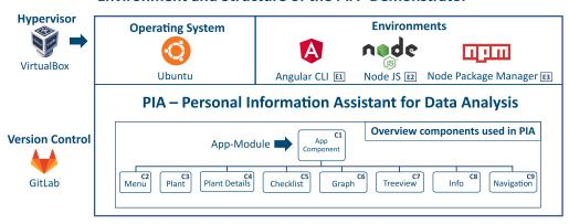
Figure 5: Schematic representation of the environment and structure of the PIA-Demonstrator.
